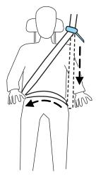
**WARNING:** Position the safety belt comfort guide so that the belt rests across the middle of your shoulder. Failure to adjust the safety belt properly could reduce the effectiveness of the safety belt and increase the risk of injury in a collision.
